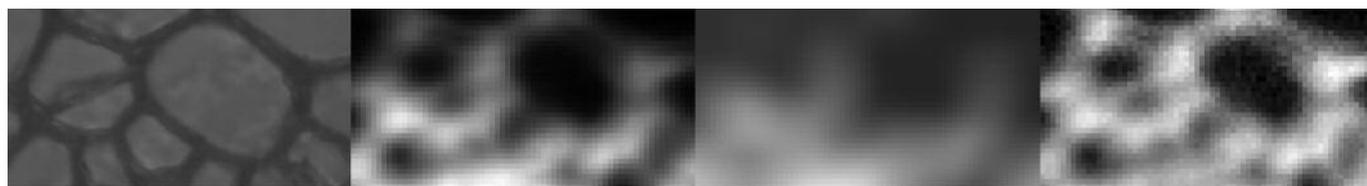
Figure 2 - a) bright field image, b) image of the sum of intensities, c) estimated shading image, d) sum of intensities after shading correction.
